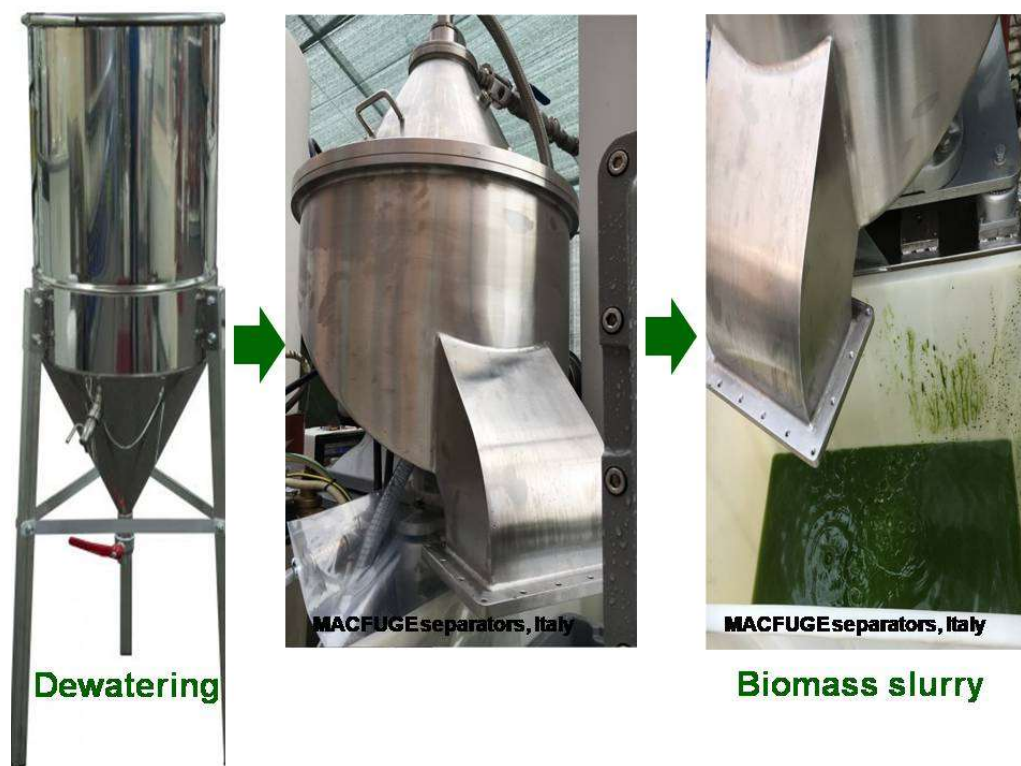
Figure 13. Harvesting process for microalgae cultures grown in open ponds or in PBRs.
