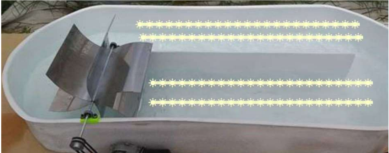
Figure 11. A model of pilot scale race way pond with internal LED illumination to support growth during shady days.
