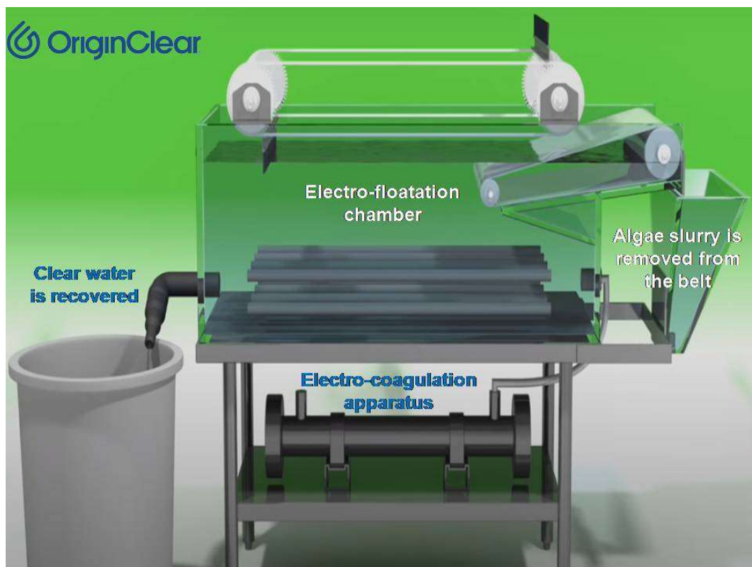
Figure 14. An electro water separation system for harvesting microalgae biomass. Source- OriginClear.
