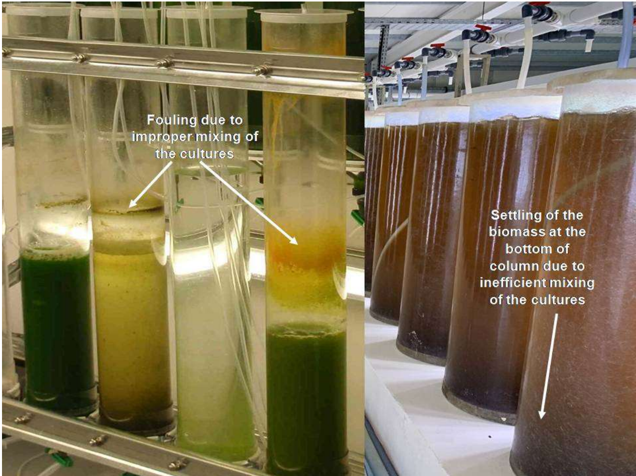
Figure 8. Air-lift column PBRs showing drawbacks of fouling and biomass settling.
